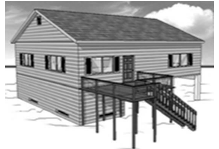
Elevated on posts, piles or piers with a properly vented partial enclosure
