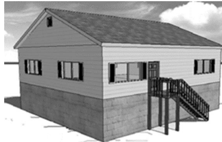
Two floor building with a full floor solid perimeter foundation for the first story and a frame construction for the second floor
